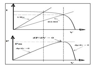
Fig.4: Working principal of any MPPT algorithm
