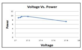
Fig.10: Voltage Vs. Power characteristics for Non-MPPT
