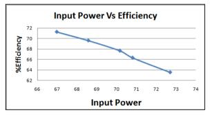
Fig.14: Input power Vs. Efficiency characteristics
