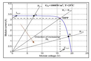
Fig.3: Solar Panel IV Curve with MPPT
