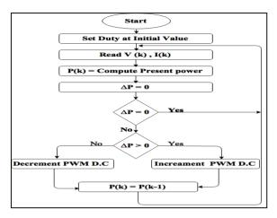
Fig.8: Flowchart of the Modified MPPT algorithm
