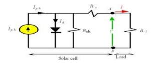
Fig.2: Equivalent Circuit of PV Solar Cell
