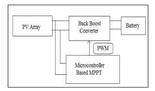
Fig.5: System Block diagram
